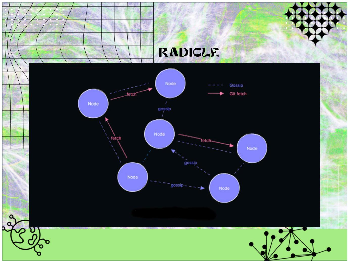
This image demonstrates the functioning of the peer-to-peer "gossip" protocol that Radicle is built upon.
